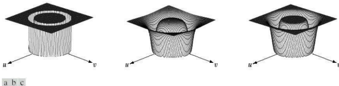
FIGURE From left to right, perspective plots of ideal, Butterworth (of order 1), and Gaussian bandreject filters.
