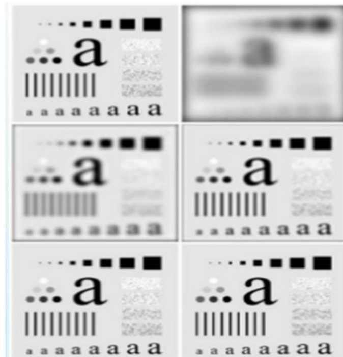
Fig. (a) Original image. (b)-(f) Results of filtering using BLPFs of order 2, with cutoff frequencies at the radii
