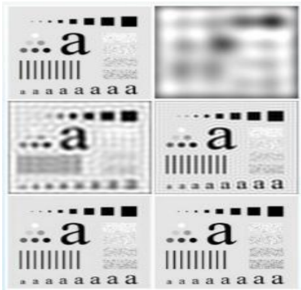
Fig: (a) original image, (b)-(f) Results of filtering using ILPFs with cutoff frequencies set at radii values 10, 30, 60, 160 and 460, as shown in fig.2.2.2(b). The power removed by these filters was 13, 6.9, 4.3, 2.2 and 0.8% of the total, respectively.
